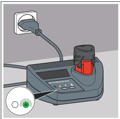
□ As soon as the green LED (right) illuminates continuously, the battery is fully charged.
