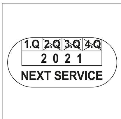
The Viega system press jaws and system press rings have a label showing the date when the next maintenance is due (e.g. 1st quarter 2021). Have your machine serviced when due to ensure safety and availability.
