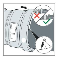
Push the press connector up to the marked insertion depth on the pipe. Do not twist the press connector.
