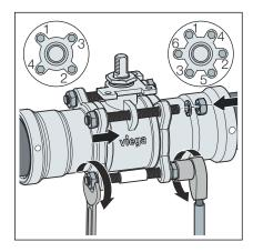
Tighten the threaded bolts by hand crosswise.
