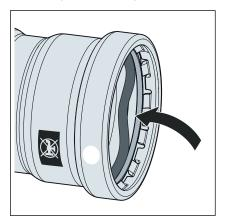
Insert a new, undamaged sealing element, model 4286XL into the bead.
