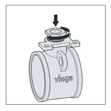
■ Tighten the stuffing box by hand.
