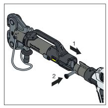
Place the Pressgun Press Booster into the press machine and push the retaining pin in until it clicks into place.
