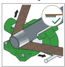
With the help of a wire brush, cleaning fleece or sanding paper, remove loose dirt and rust particles from the pressing area.
