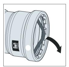
Remove the sealing element from the bead. Proceed carefully to avoid damaging the sealing element seat.
