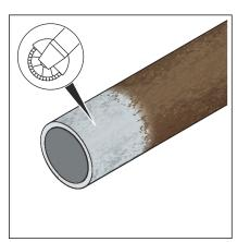
Angle grinder with serrated washer
