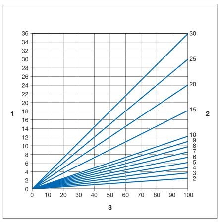
Fig. 3: Length expansion steel pipes
