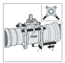
Grease the threaded bolts and insert using the centering aids.
