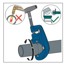
Cut the pipe at a right angle using a pipe cutter, angle grinder or fine-toothed hacksaw. Do not use a flame cutter
