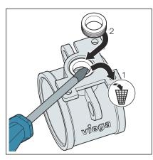
**NOTICE!** The seal cannot be removed without being destroyed. Before you remove it, check whether a spare seal is available.
