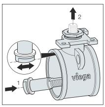
Insert the selector shaft with the new seal from below.
