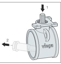
Push out the selector shaft from top to bottom.
