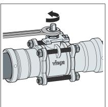
Loosen the stuffing box with a fork spanner.
