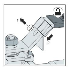
The ball valve can be secured against accidental and/or unauthorized operation.
