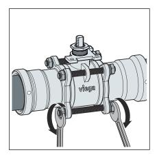
Loosen the flange connections.
