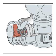
Triggered TSS can no longer be opened and are no longer fit for use.
