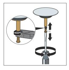
Set the valve cone with the help of the adjusting screw and counter with the nut.
