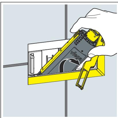
► Remove the drain valve through the revision opening.
