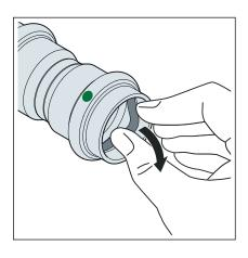
Remove the sealing element from the bead.
