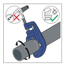
Cut the pipe at a right angle as accurately as possible using a pipe cutter, an angle grinder or a fine-toothed hacksaw to ensure a complete and even pipe insertion depth. Do not use a flame cutter.
