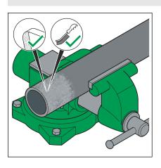
With the help of a wire brush, cleaning fleece or sanding paper, remove loose dirt and rust particles from the pressing area.
