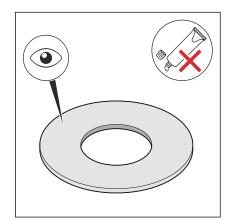
The seal must be clean, undamaged and dry. Do not use adhesives and assembly pastes for seals.
