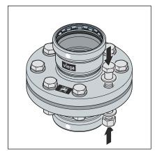
The simultaneous use of several tightening tools is possible.
