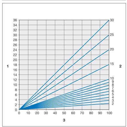
Fig. 3: Length expansion steel pipes
