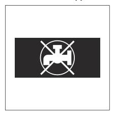
The system is intended for use in industry, heating and cooling systems and is a replacement for weld, threaded and roller-groove connections during new installations and repairs. The system is not suitable for use in potable water installations. For this reason, the press connectors are labelled with a black symbol "Not potable water".
