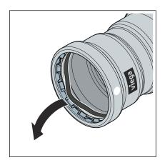
Remove the sealing element from the bead. Proceed carefully to avoid damaging the sealing element seat.
