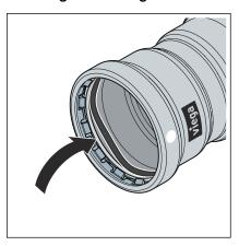
Insert a new, undamaged sealing element, model 4286XL into the bead.
