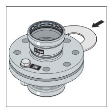
The correct assembly of flange connections requires parallel aligned flange blades without an offset centre that allow the sealing element to be inserted in the correct position without damage.
