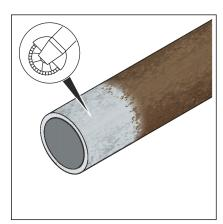
Angle grinder with serrated washer
