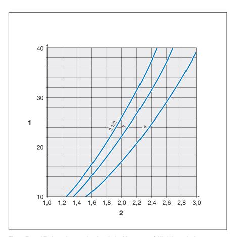
Fig. 5: Z- and T-shaped expansion bends for Megapress S XL 2% to 4 inches
