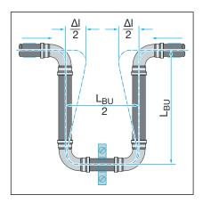
Fig. 6: U-shaped expansion bend
