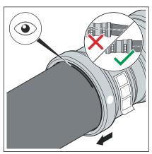
Push the press connector up to the marked insertion depth on the pipe. Do not twist the press connector.
