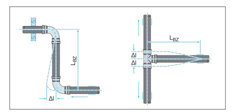
Fig. 4: Z-shaped and T-shaped expansion bends
