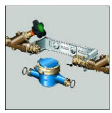
Loosen the fixing nut of the slide and push in the slide.
