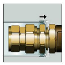
Screw the lock nut finger-tight against the water meter bow.
