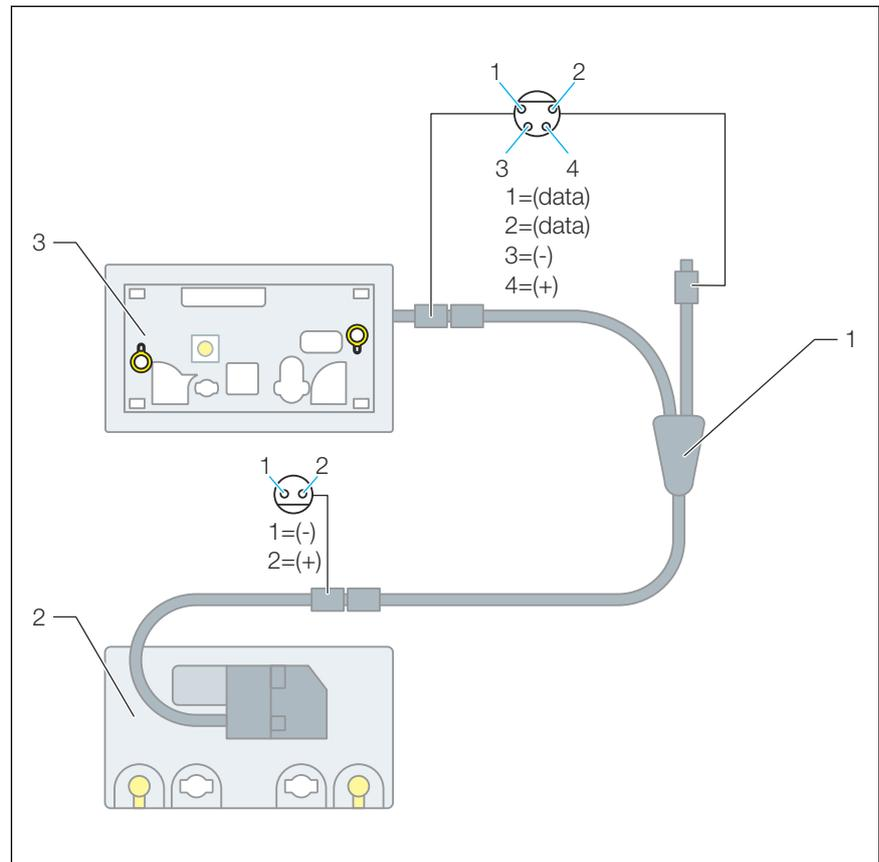
**Fig. 2: Connection diagram, WC installation frame for Prevista**
