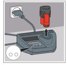
When the battery is fully charged, the charger automatically switches to trickle charge. There is no danger of the battery becoming overcharged.
