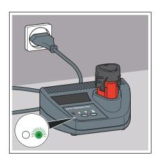
$\,\square\,$  As soon as the green LED (right) illuminates continuously, the battery is fully charged.
