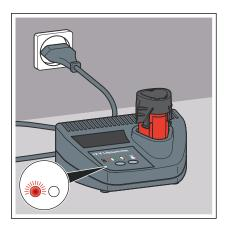
The red LED (left) illuminates continuously when the battery is charging.
