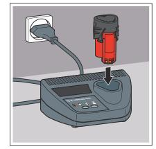
Insert a 12 V battery into the battery compartment of the charger.
